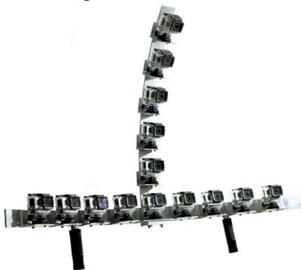
Figure 11: GoPro Rig Curved Vertical Element – Cameras
