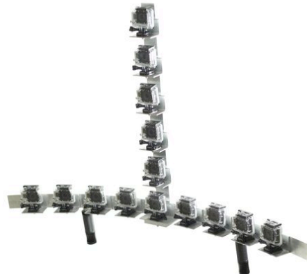
Figure 13: GoPro Rig Straight Vertical Element – Cameras
